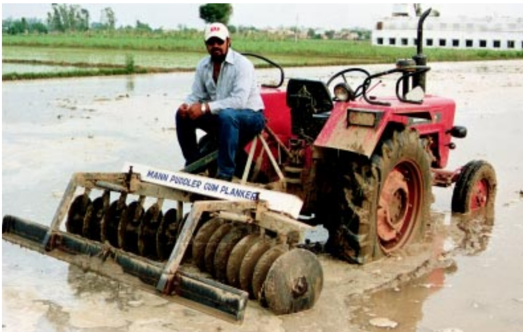
An innovative and progressive farmer from Karnal, Haryana, with his puddler-cum-planker which saves energy and facilitates good puddling and leveling.
