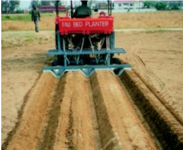
A bed-planter of the Punjab Agricultural University in operation in one of its fields.
