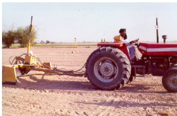
Laser Leveler being used in Haryana
