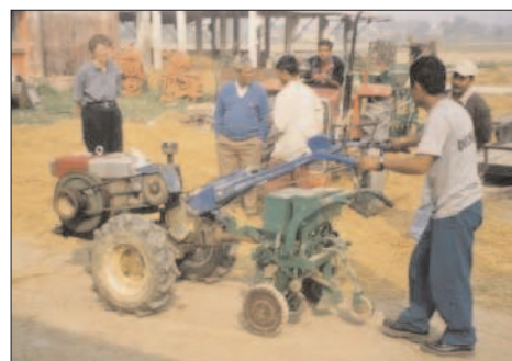
Animal drawn zero-till drill being hitched with CHT in Bangladesh
