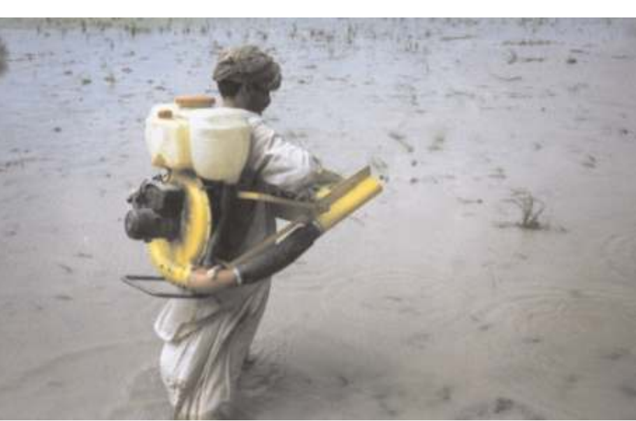
Fig. 7. Power blower modified for broadcasting seedlings.
