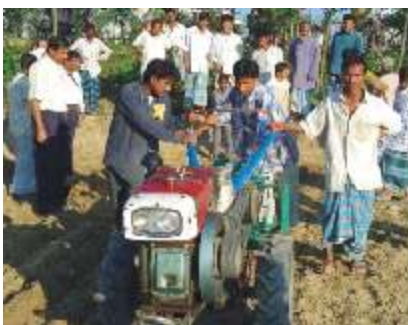
2-wheel tractor compatible potato planter attachment in Bangladesh means its reach to major farmers there for crop diversification
