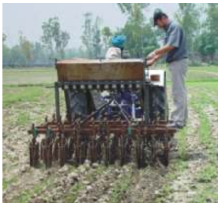
Double disk planter: Wheat planted with double disk drill in the residues of lodged rice crop (a) and field a month after sowing (b).
