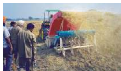
Figure 1. The chopped material is dropped directly behind the drill as mulch on the seedbed.
